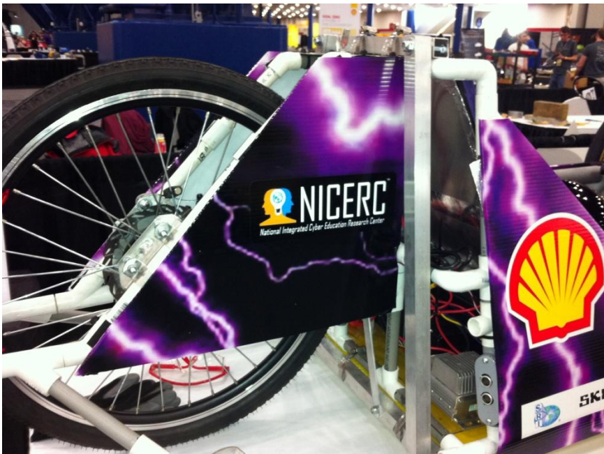
The Eco-Tiger prototype uses an electric hub motor, motor controller, and Lithium Ion battery for propulsion, which came from Electric Bike Solutions, LLC in California.
